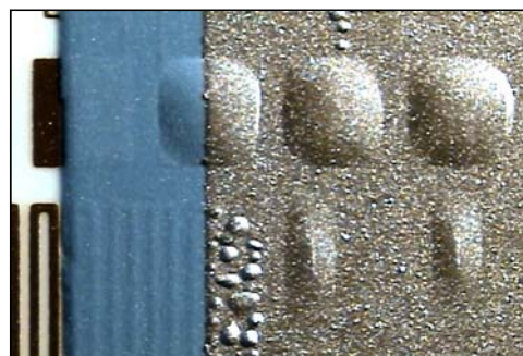
Figure 2: Battery effect after 3 firings (850 °C). Bottom electrode: Au, blue layer: dielectric, top electrode: Ag/Pt Figure 3 shows the test results of IP9227 for the battery effect after 12 refirings @ 850 °C. There is no formation of bubbles visible. The Fired Film Thickness (FFT) of electrodes was 12 µm, the thickness of the dielectric between 35 – 40 µm (FFT).
